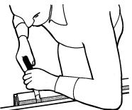
N.B. Keep all parts of the body behind cutting edge.
