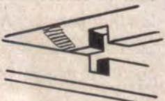
Cross Half Lap. A good strengthener where two square pieces cross each other.
