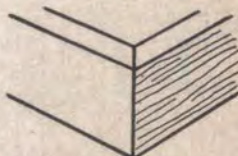
Mitre Joint. Usually cut at 45° but may be varied to any angle.
