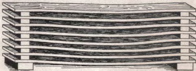
Fig. 4B. Showing spacers placed too far apart with consequent sagging and eventual bad warping if the boards stand for any length of time.
