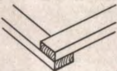
Half Lap Splice. For joining the ends of two straight or curved pieces to lengthen a member.
