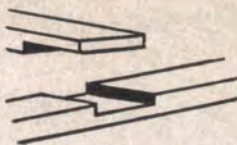
Middle Half Lap. The ideal T-joint as for dividing cross members to a main frame.
