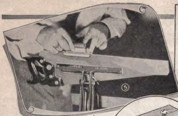
VICE FOR HOLDING CIRCULAR SAW AND DADO HEAD WHEN FILING
