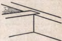
Dado Joint. A grooved joint cut across the grain.
