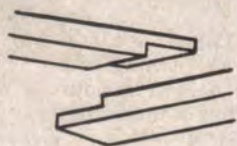
Mitred Half Lap. For same uses as end half lap but gives greater bracing.
