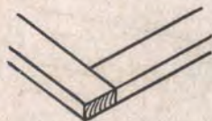
Plain Lap Joint. Commonly used for splicing, angling, or corner lapping.
