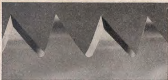
Fig. A—Side view of hand crosscut saw showing correct angle and amount of bevel, appearance of points, also smoothness and evenness of gullets.
