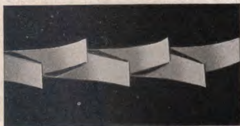
Fig. C—Side view of Rip Saw showing correct smoothness of faces, points, and gullets.
