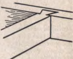
End Dado Joint. Combines the dado and rabbet joint. Can be varied by making a tongue-and-rabbet dado.
